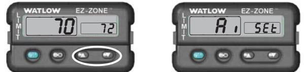
**Setup Page from Home Page:** Press both the Up ▲ and Down ▼ keys for six seconds.
