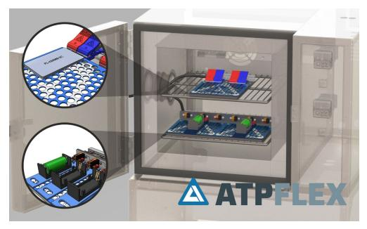
You get the flexibility to test battery cells in any quantity, any style, and any size in an environmental test chamber that you already own.
